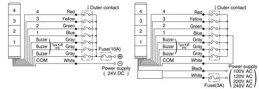
\* This wiring diagram is for the four-light unit. The number of signal wires will vary for other number of lights (Refer to Table 1.)
