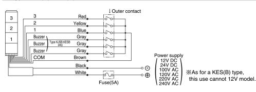
\* This wiring diagram is for the three-light unit. The number of signal wires will vary for other number of lights (Refer to Table 1)
